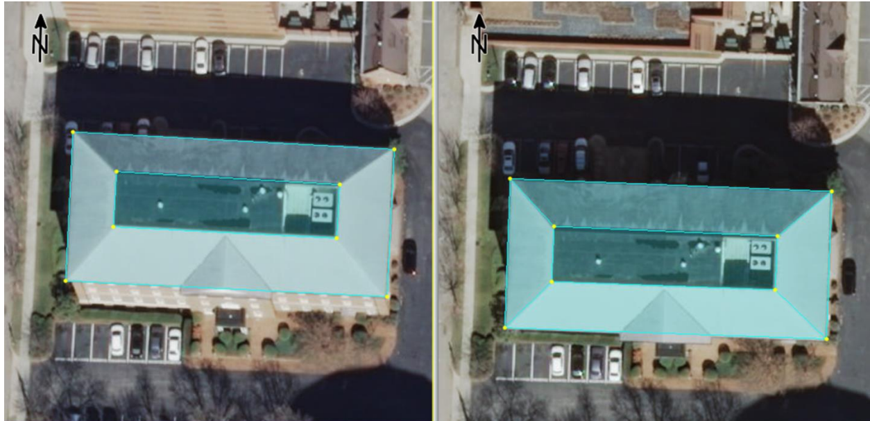
Figure 53. Loft a polygon to another polygon to create a truncated pyramid.
