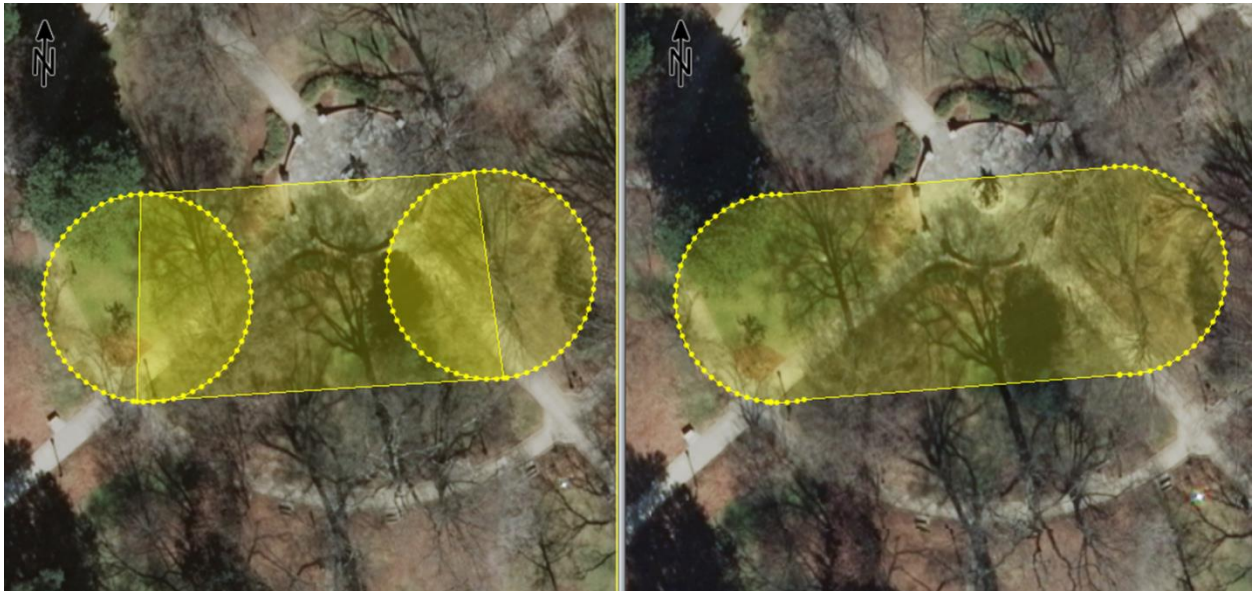
Figure 55. Combining multiple shapes using Boolean geometry.
