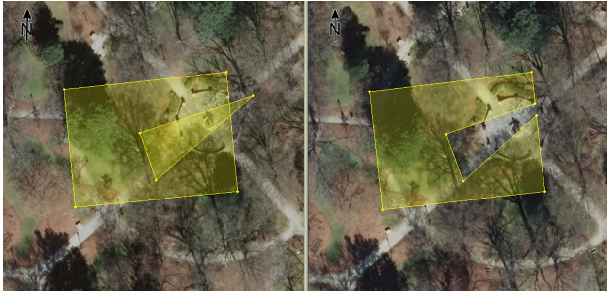
Figure 56. Using Boolean subtraction to carve complex shapes.
